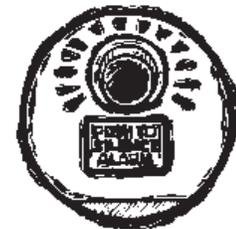
**Do** remember that the audible alarm can be silenced by pushing the lighted button located directly above the "Push to Silence" label on the front of the electrical control panel. Hold the button until the alarm goes off. With normal use, the tank has a reserve storage capacity good for about 24 hours.
